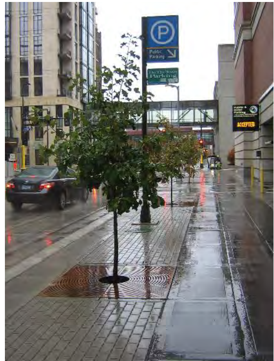
Downtown Trees Planted within Underground Stormwater Cells
