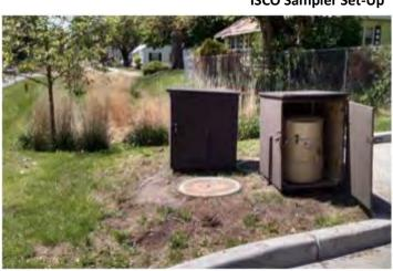
**ISCO Sampler Set-Up**
