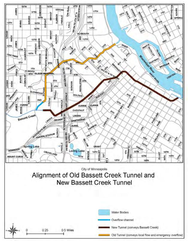
Figure 3.9 – Original and New Bassett Creek Alignment
