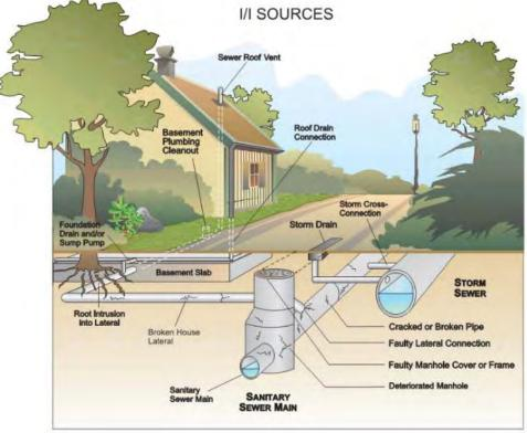
Figure 4.9 – Typical Sources of Inflow/Infiltration
