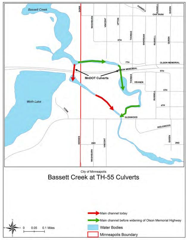
Figure 3.8 – Bassett Creek Culverts at Trunk Highway 55
